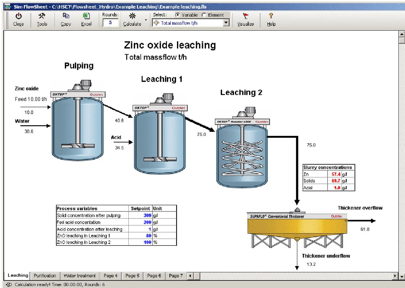
HSC 7 has multiple **new high-resolution icons** for different unit processes. The unit icons are grouped under the following folders: Acid Plan, Analyzers, Experimental, Ferro, Flotation, General, Grinding, H2SO4, Hydro, Iron&Steel, Minerals-Others, Others, Physical Separation, Precious Metals, Pyro, Roasting, Thickeners.
